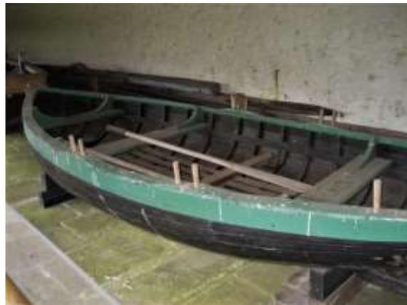
Occasionally, Llangwm boats carried a short mast which was stepped through the forward thwart (seat). This would have carried a small lugsail. With no depth of keel or centreboard, this sail would have been mainly used when the wind was astern or over the aft quarter.
