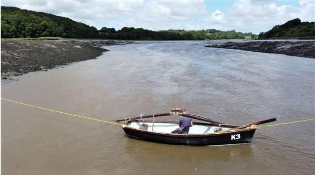
*As the tide approaches the last of the ebb, the boat is secured fore and aft to lie across the channel.*
